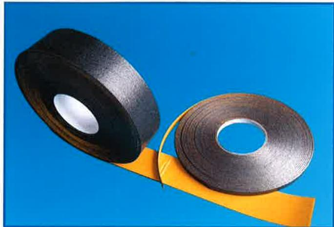
The mode of action is based on the forming of a temperature-reducing foam in case of fire. Joints, gaps and other openings will be filled by the formed foam and prevent the conductivity of temperature.
